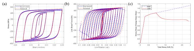
Figure 4. (a) Calibration of Giuffré-Menegotto-Pinto material model (data by Dehghani et al. 2016 [18]); (b) Shear forceshear deformation beahaviour of the W250x28 link (data by Okazaki et al. [21]); (c) Lateral force-lateral deformation response.
