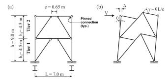
Figure 2. (a) Geometry of the selected two-tiered EBF; (b) Expected plastic mechanism of two-tiered EBF with shear links under seismic loads,  $\theta$  = tier plastic rotation  $\Delta$  = tier lateral deflection (deformations and rotations shown for Tier 2 only).
