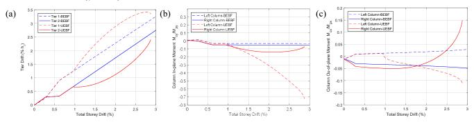
Figure 5. (a) Tier drifts; (b) Column in-plane bending moments; and (c) Column out-of-plane bending moments.
