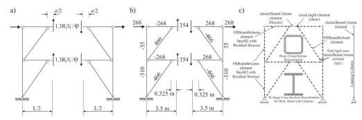
Figure 3. (a) Probable link resistances; (b) Capacity-induced seismic forces under the probable link resistance (forces in kN); and (c) Numerical model of the two-tiered eccentrically braced frame.
